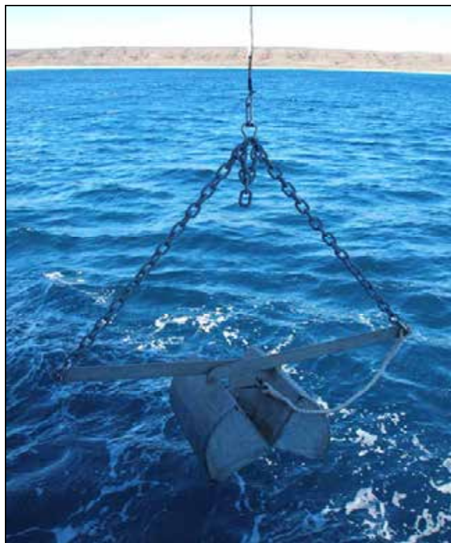
Figure 4. Van-Veen grab sampler for collecting surface and subsurface material to a depth of ~10 cm from Ningaloo Marine Park.
