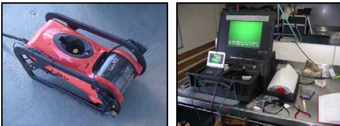
Figure 21. a) LBV ROV Seabotix remote operated vehicle. b) ROV operating console.
